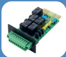
DRY CONTACT Contactos seco
